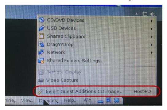
Click on [Device] and then select [Insert Guest Additions CD image...]. After downloading and installation is complete, access the CD drive device from your operating system. You should be able to see a screen similar to the one shown in the graphic below.
