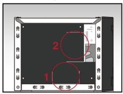
2. For both memory modules, pull back the black protective covering, and then release the ejector clips by gently pulling them out to the sides. Remove the memory modules.
