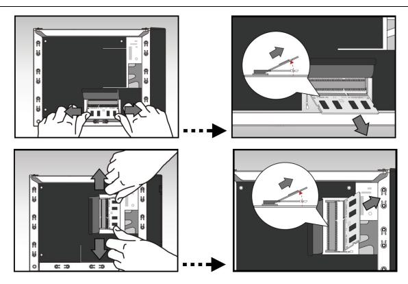
3. Diagonally slide the new memory module into slot No.1 (as shown in the graphic below) making sure that the memory module's connectors are fully inserted into the slot. Using two fingers, carefully push down and then back on the memory module until it clicks into place. You should be able to hear an audible "click".
