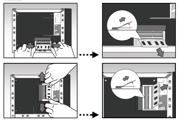
3. For each slot, diagonally slide in a new memory module (as shown in the graphic below) making sure that each memory module's connectors are fully inserted into the slot. Using two fingers, carefully push down and then back on the memory module until it clicks into place. You should be able to hear an audible "click".
