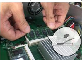
2. Using two fingers, carefully push down and then back on the memory module until it clicks into place. You should be able to hear an audible "click".
