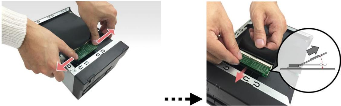
3. Diagonally slide the new memory module into slot No.1 (as shown in the graphic below) making sure that the memory module's connectors are fully inserted into the slot. Using two fingers, carefully push down and then back on the memory module until it clicks into place. You should be able to hear an audible "click".
