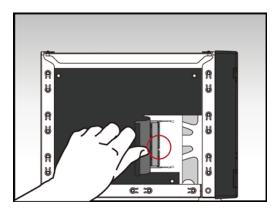
• Diagonally slide in the memory module (as shown in the illustration) making sure that the memory module's connectors are fully inserted into the slot.
