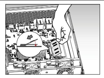
• Using two fingers, carefully push down and then back on the memory module until it clicks into place. You should be able to hear an audible "click".
