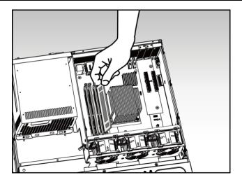
• Using two fingers, carefully push down on the memory module until the ejector clips lock it into place.
